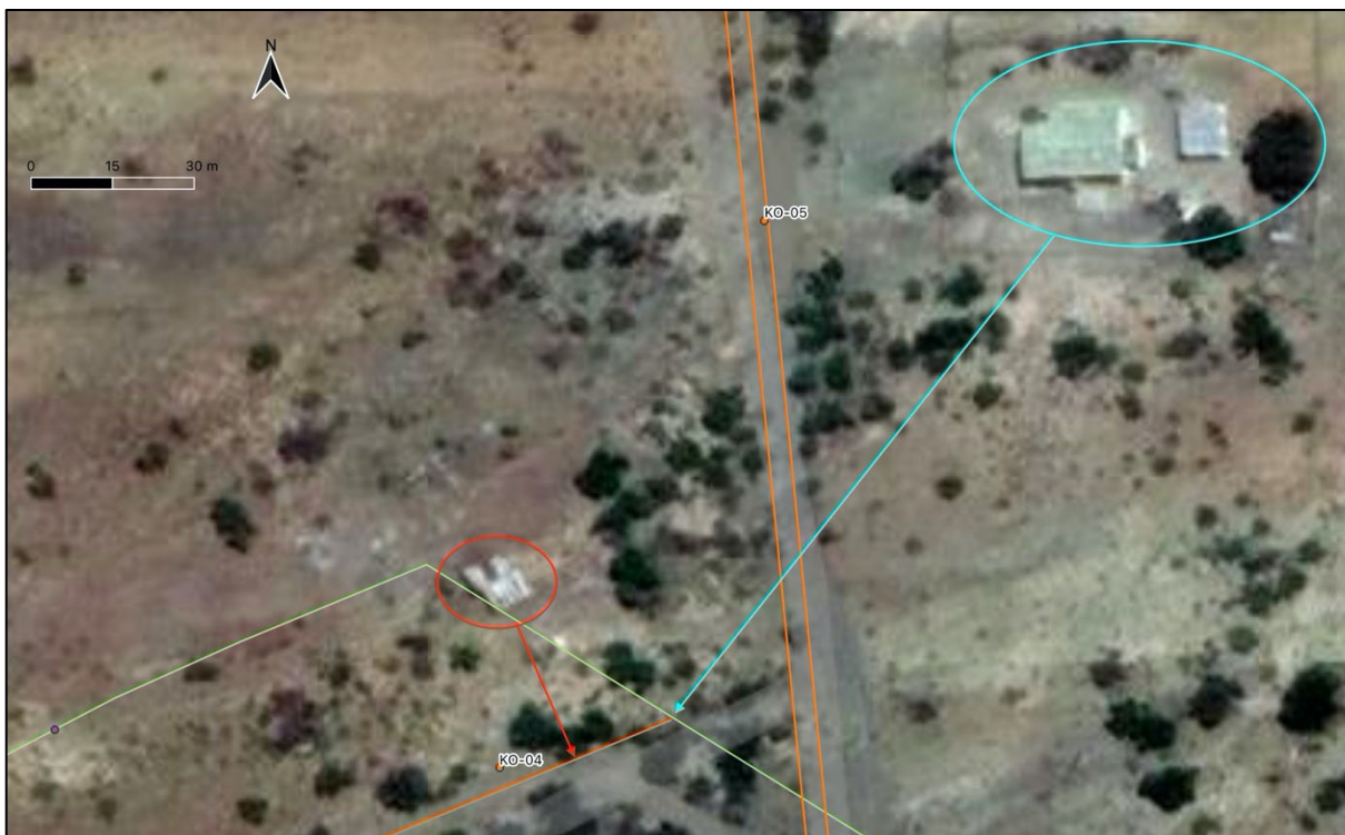
Figure 4: Proximity of access road (orange line) and OHPL (green line) to modern labourers' cottage KO-04 (red circle). The cottage is approximately 25 m from the current roadway (red arrow) and will not be affected by the roadway upgrade, but the proposed OHPL appears to pass directly over the structure. Note also the location of the Platdorings farm complex (KO-05) approximately 100 m from the access road and OHPL.
