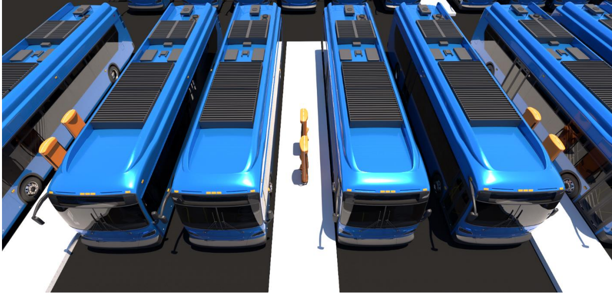
Figure C-8 Depot Charging with ground-mounted CCS corded chargers
