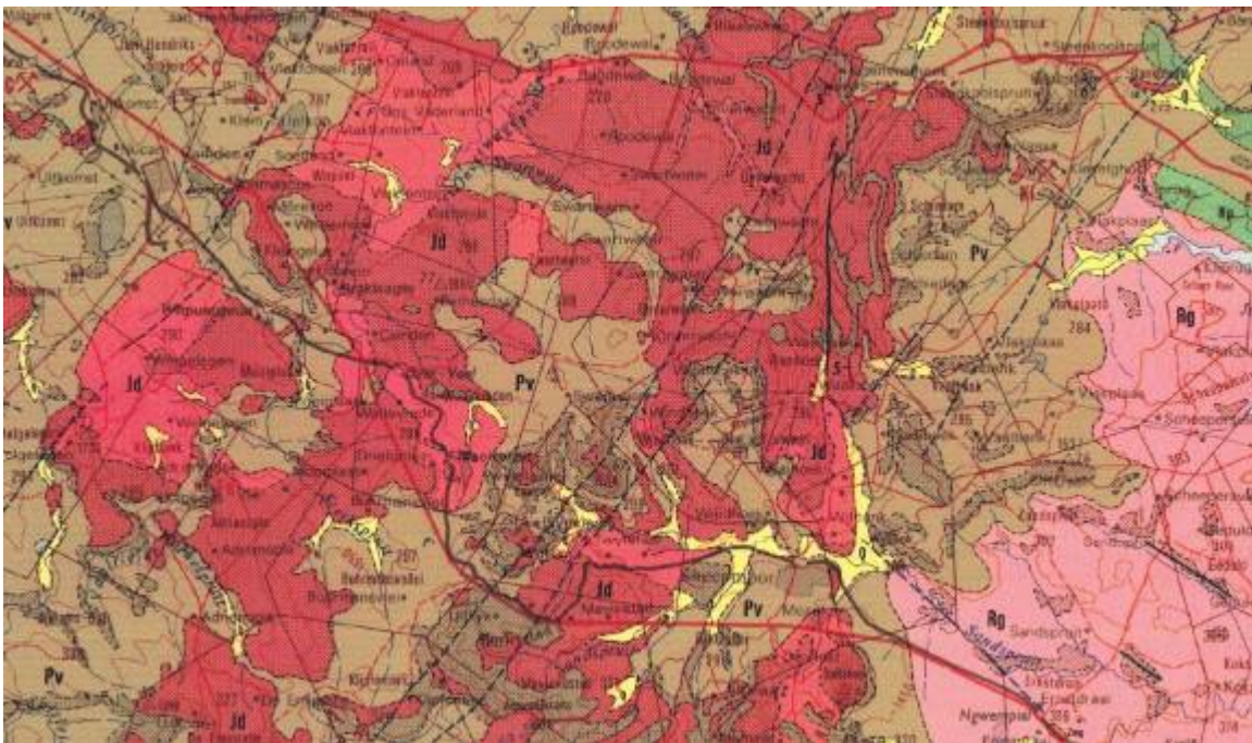
Figure 3: Extract from the Mbabane (2630) 1:250 000 Geological map. According to this map, the proposed Camden WEF Development site is underlain by Vryheid Formation (Pv: grey) and Karoo Dolerite (Jd: red).
