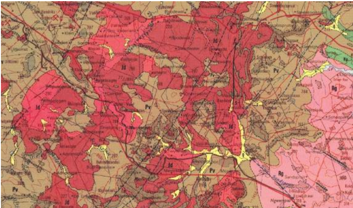
Figure 3: Extract from the Mbabane (2630) 1:250 000 Geological map. According to this map, the proposed Camden WEF Development site is underlain by Vryheid Formation (Pv: grey) and Karoo Dolerite (Jd: red).
